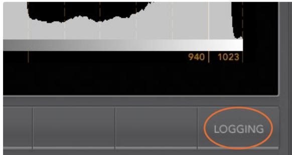
From the Histogram Display, select the Logging button to switch to the Error Logging Display.
