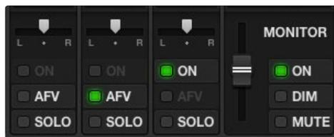
The monitor fader and checkboxes set independent audio levels and allow solo monitoring on the audio output.
