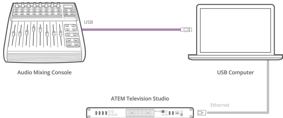
You can adjust multiple audio levels at the same time by connecting a hardware audio mixer to the computer which is running ATEM Software Control.
