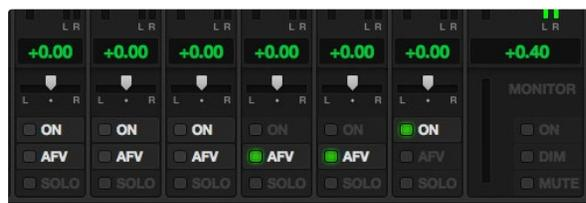
If you are operating an ATEM 1 M/E, 2 M/E or Production Studio 4K and notice the solo and monitor settings are grayed out, you have program audio selected for the audio out setting in the settings tab. The solo and monitor settings are always grayed out on ATEM Television Studio.
