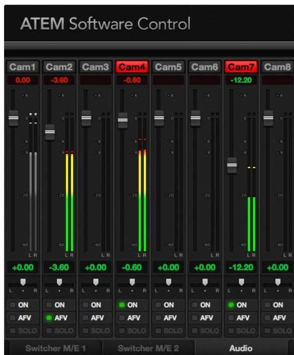
The audio mixer displays red tally lights for any audio sources that are currently on air, as well as audio level, audio balance and checkboxes for selecting which audio should be used.
